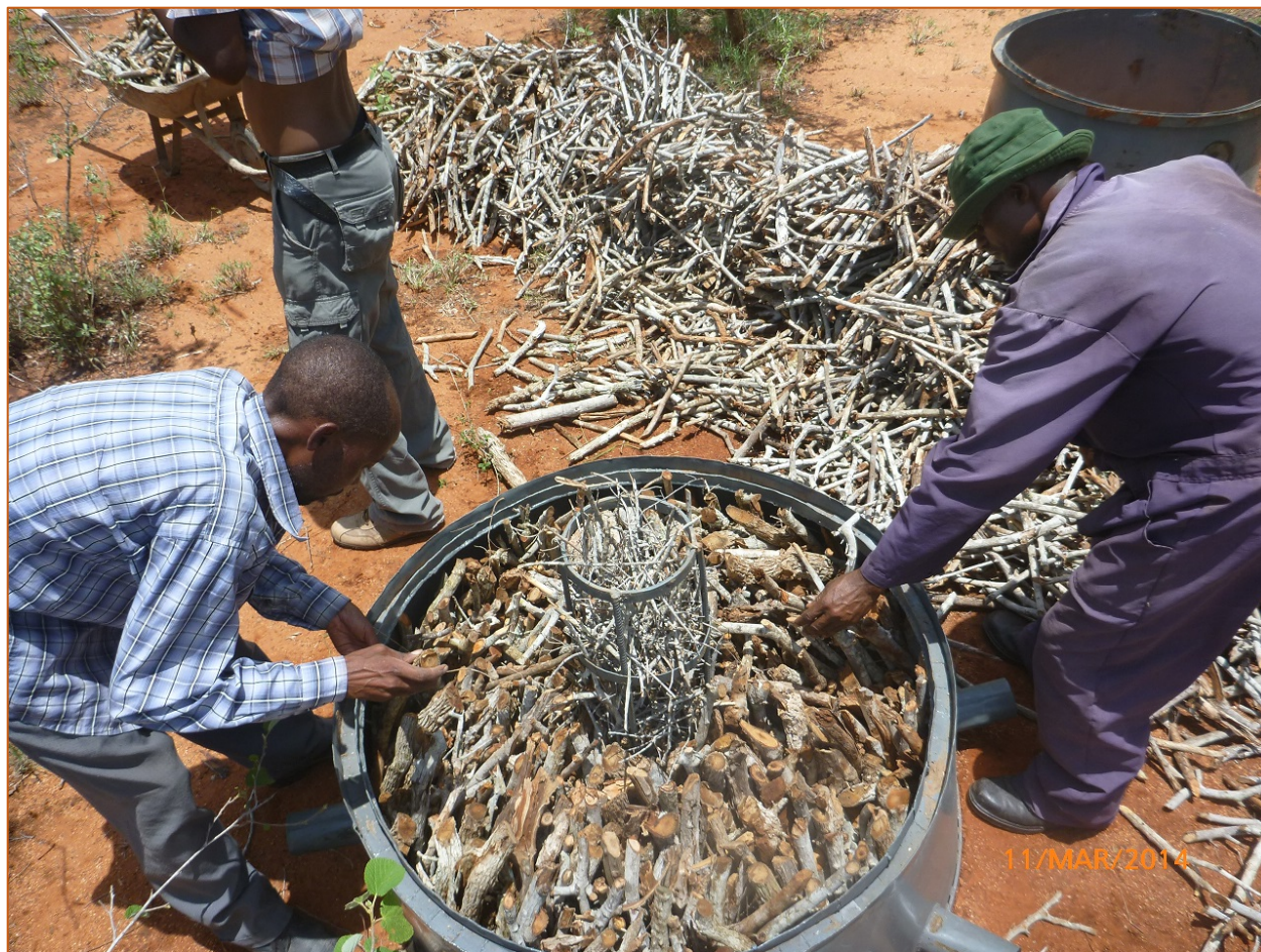
Figure 27: Setting up a test kiln at the new eco-charcoal production site
